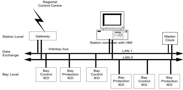
System Architecture of Substation Automation
