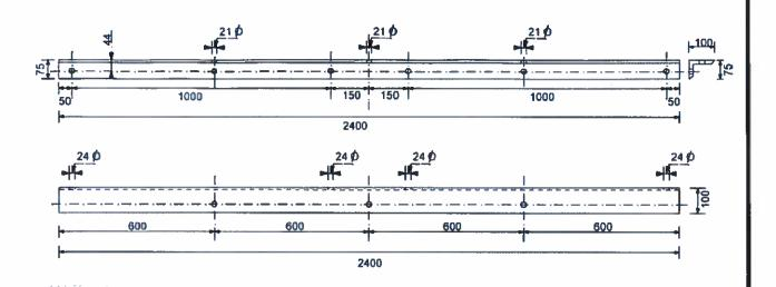
FIG. 9: 33kV CROSS ARM: <u>KPLC CODE 182960</u> (L2400mm x 100mm x 75mm x 9.5mm structural steel angle, galvanized)
