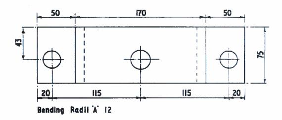
FIG. 14: BRACKET INSULATOR - HV, - (structural steel, galvanized) CODE 186947
