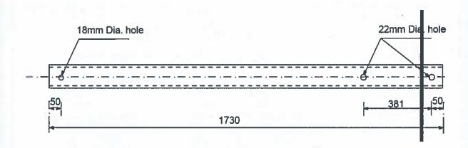
FIG. 7: EARTH STOCK: KPLC CODE 186928 ('U' Channel 1730mm x 100mm x 50mm x 6mm structural steel, galvanization.
