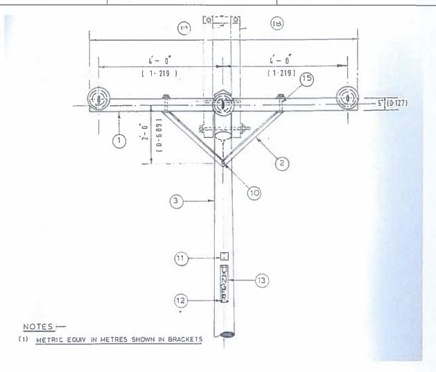
FIG. 17: APPLICATION OF 33KV ANGLE TIE STRAP (item 2 in drawing, shown with wooden cross-arm - same item used on steel cross-arm)
