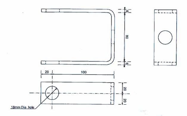
FIG. 1: D – IRON (LV Insulator Bracket): <u>KPLC CODE 181201</u> (332mm x 40mm x 6mm structural steel, galvanized)
