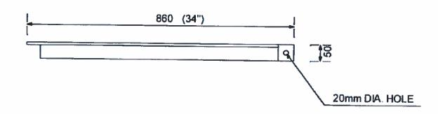
FIG. 4: 33KV TIE STRAP: KPLC CODE 188108 (860mm x 50mm x 50mm x 6mm structural steel angle, galvanized)
