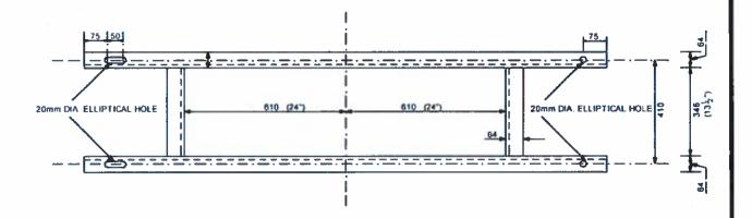
FIG. 13A: TRANSFORMER PLATFORM 315 KVA <u>KPLC CODE 186924</u> (1980mm x 125mm x 64mm x 6mm structural steel, galvanized) (To be complete with mounting brackets in Fig. 13B)
