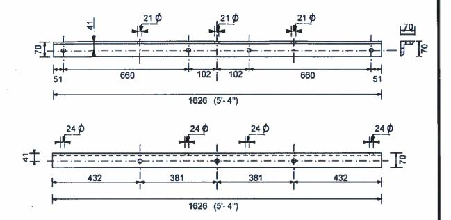
FIG. 8A: 11KV CROSS ARM: <u>KPLC CODE 182911</u> (L1625mm x 70mm x 70mm x 9.5mm structural steel angle, galvanized)
