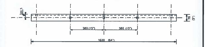
FIG. 8B: 11kV TERMINAL CROSS ARM: <u>KPLC CODE 182914</u> (L1620mm x 125mm x 76mm x 9.5mm structural steel angle, galvanized)
